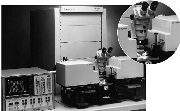
8510XF configured with a wafer probing station and 1.0 mm probes
