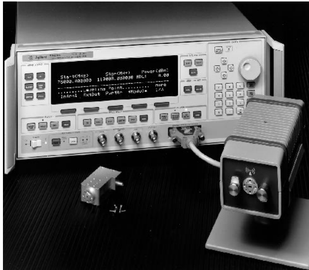
83558A mm-wave source module. 75GHz to 110 GHz
